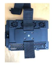
Align 4-hole pattern with X-naut and inster 8-32 screws.
