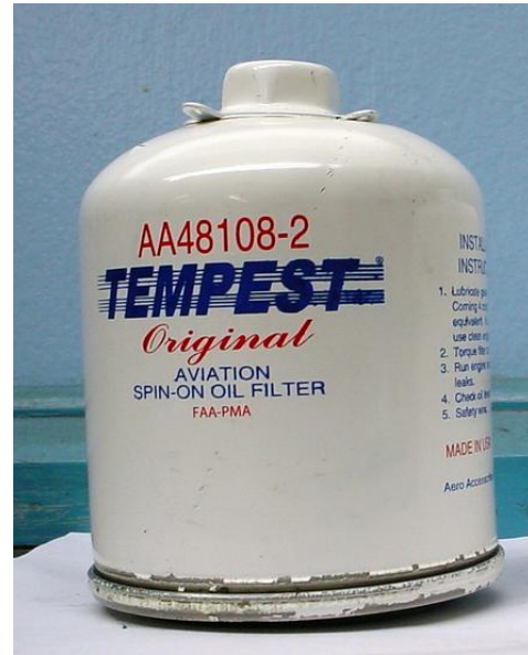
FIGURE 3 BURST FILTER CASE FROM OVERPRESSURE
