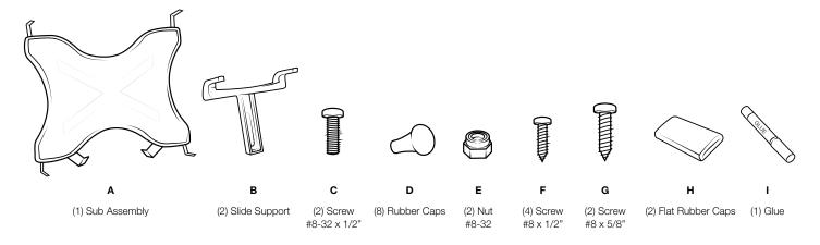
1 Attach (D) and (H) Rubber Caps to each prong on (A) Sub Assembly. Use optional (I) Glue for a secure hold.
