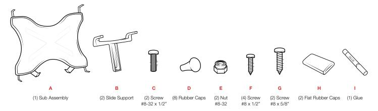
1 Attach (D) and (H) Rubber Caps to each prong on (A) Sub Assembly. Use optional (I) Glue for a secure hold.
