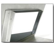
Drill the 4 holes in the rail for an 8-32 screw — recommended drill size is #16.
