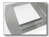
You will need a cutout in the Panel of approximately 8.00" x 6.43". If you opt for a tighter fit, make sure the angle adapter does not deform when placed in the opening. Next, install support structures on the sides such as aluminum angles (rails). Once you have prepared the panel and installed the rails you can continue with this document.
