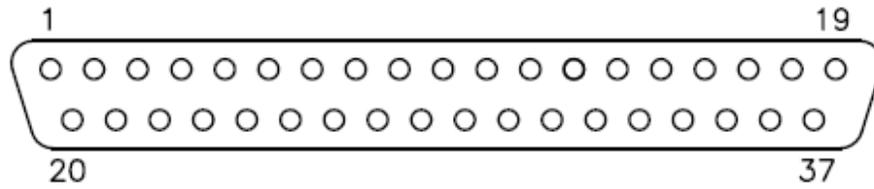
**Figure A-6 GEA 24/GEA 24B J243/P243 Connector (Looking at Unit)**
