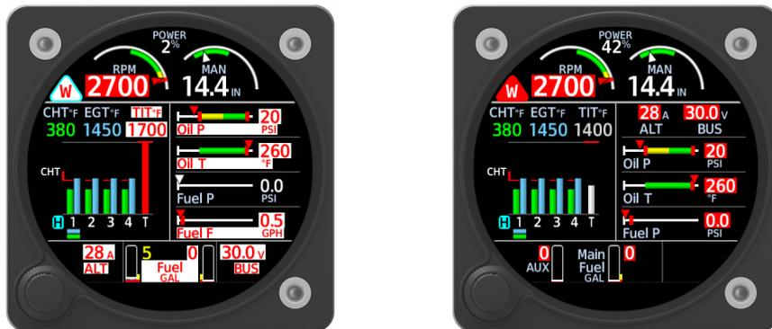
Figure E-18 Warning Alert (Flashing and Acknowledged)
