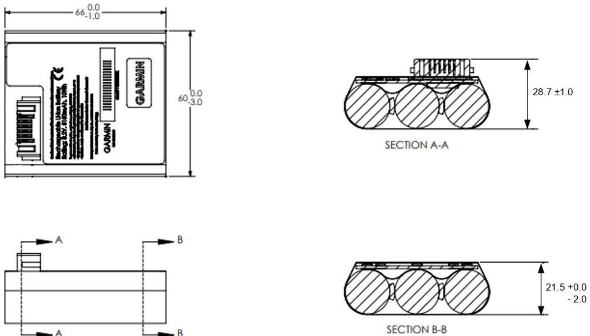
**Figure 4-9 Backup Battery Dimensions
