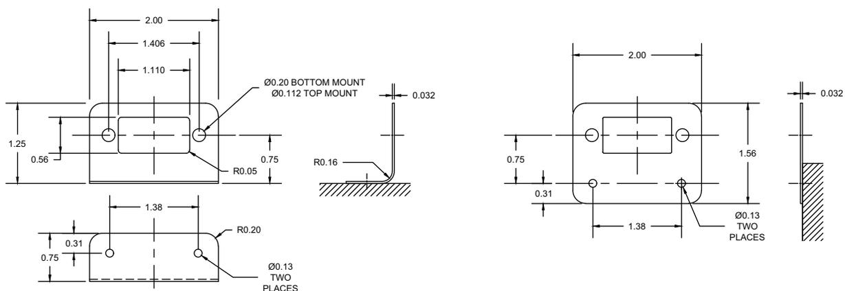
Figure 4-42 10A Relay Bracket Examples
