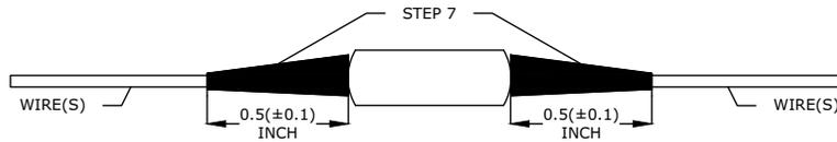
NOTE: DURING THE HEAT SHRINKING PROCESS ENSURE THE RESISTOR IS MINIMALLY EXPOSED TO DIRECT HEAT.
