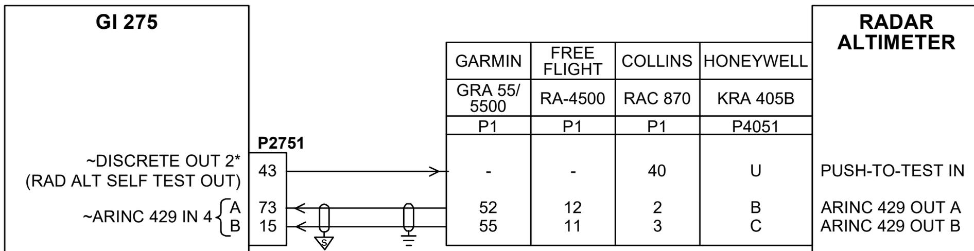
Figure B-10 Radar Altimeter Interconnect
