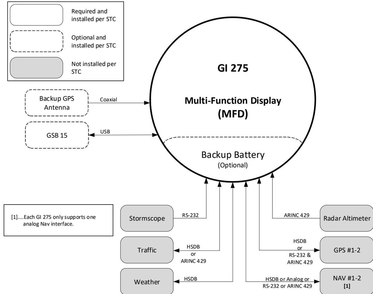
**Figure 1-2 GI 275 Multi-Function Display Indicator**
