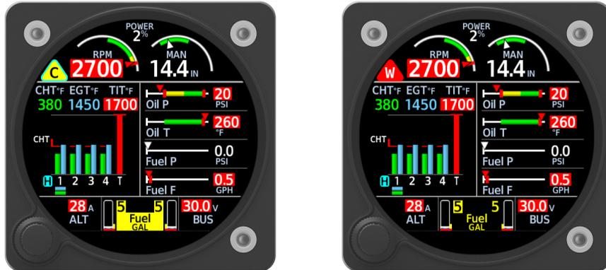
**Figure E-20 New Caution Alert with Ongoing Warning Alert**
