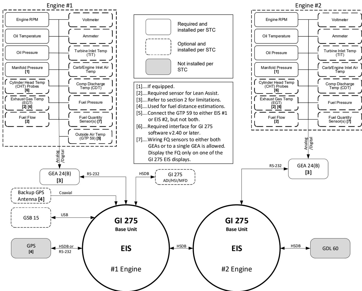
Figure 1-5 GI 275 Twin-Engine EIS Interfaces
