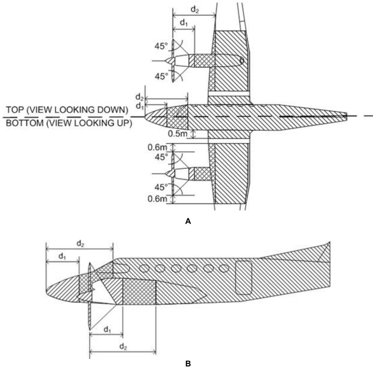
**Figure F-10 Zoning for Front-Mounted Twin Propellers (Low- or High-Wing)**
