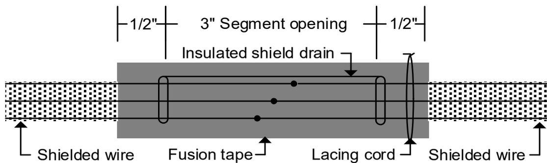
**Figure F-1 Shielded Wire Splice**
