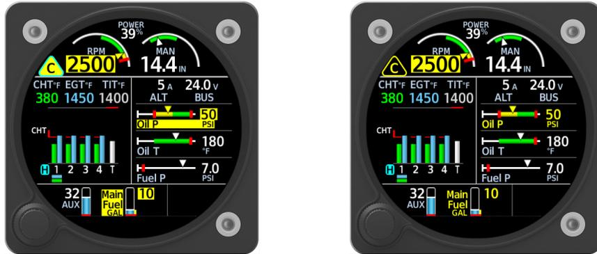
Figure E-17 Caution Alert (Flashing and Acknowledged)
