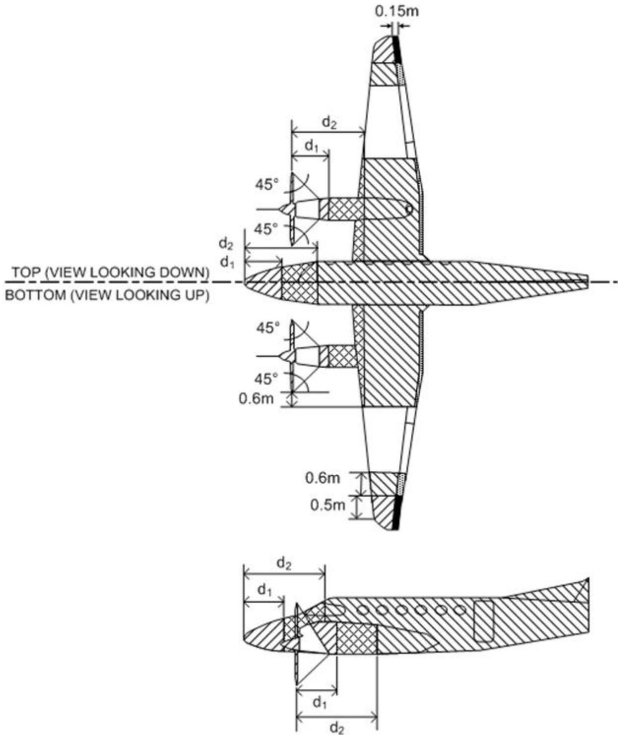
Figure F-20 Example Lightning Zoning for Twin-Engine Aircraft
