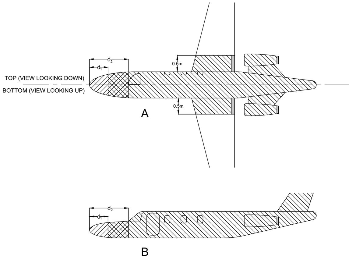
Figure F-17 Single Jet Engines with Two Inlets Zoning, Low or High Wing
