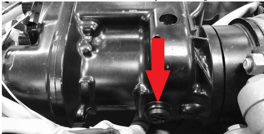
Figure 4-40 TCM/Bendix Magneto Vent Hole
