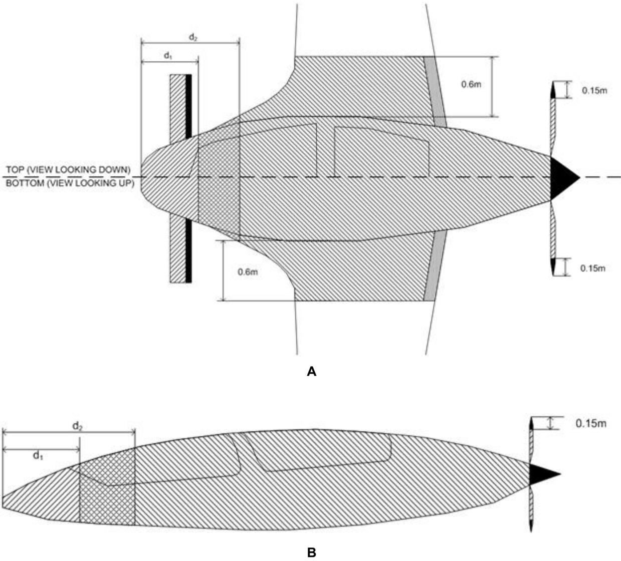
**Figure F-7 Zoning for a Low- or High-Wing Canard with a Rear-Mounted Propeller**
