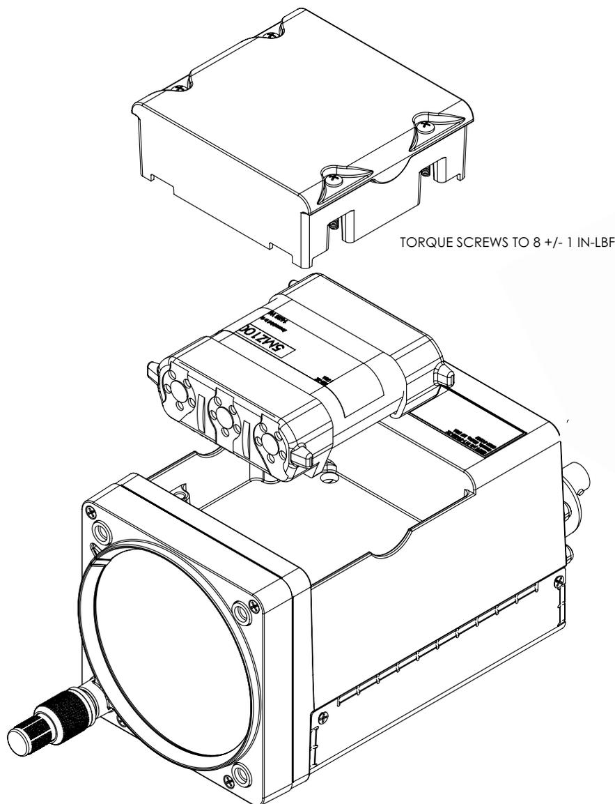
**Figure 4-10 GI 275 Backup Battery Installation**
