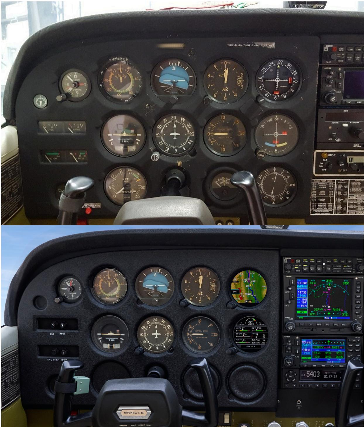
**Figure 1-1 GI 275 System Installation (Before and After Example)**
