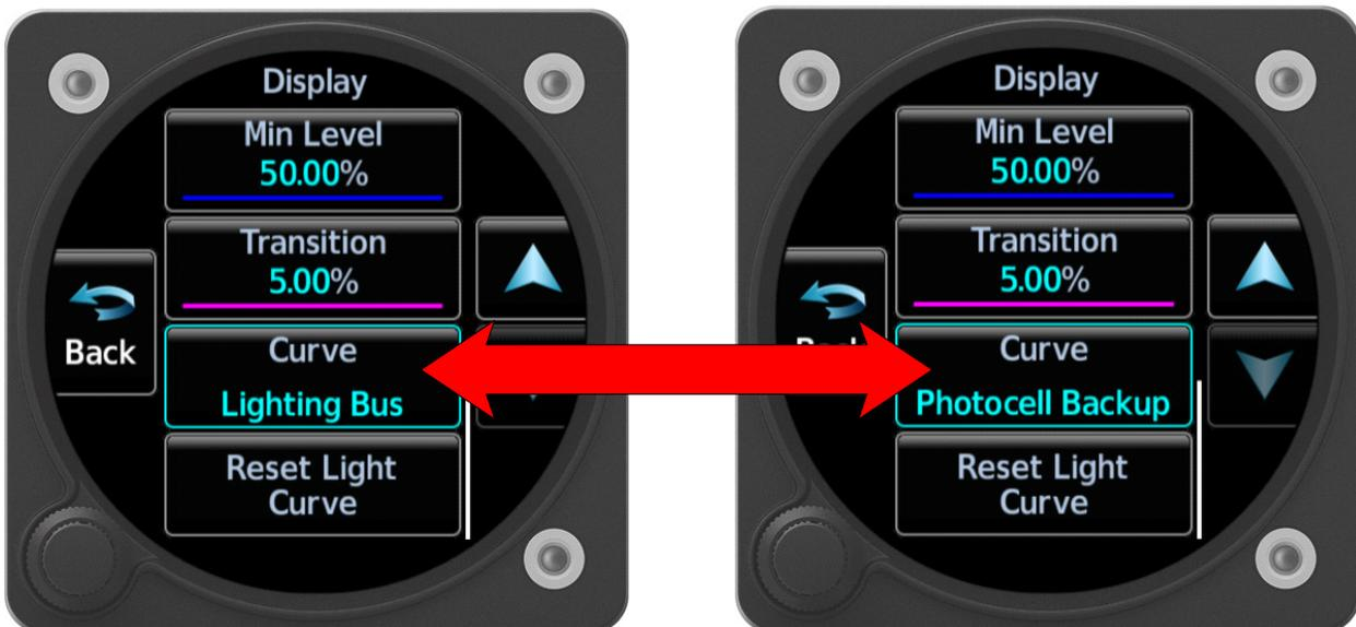
Figure 5-11 Selection Between Lighting Bus and Photocell Backup Curves
