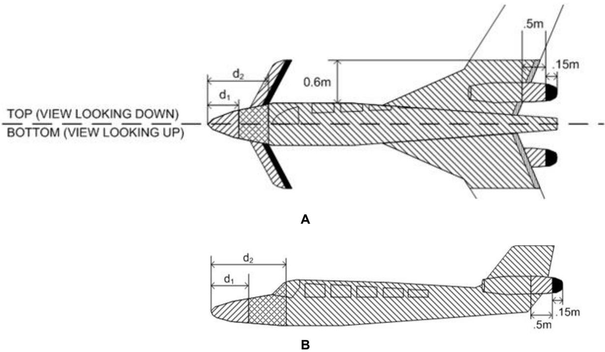
Figure F-14 Zoning for Low- or High-Wing Canard with Twin Jet Engines
