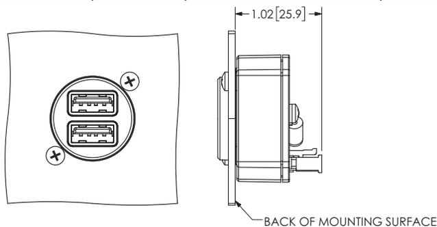
SIDE CONNECTOR (-01, -30, -50), WITH CONNECTOR KIT (011-05044-00)
