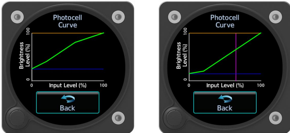
Figure 5-9 Enhanced Lighting Mode Example Photocell Display (Left) and Knob (Right)
