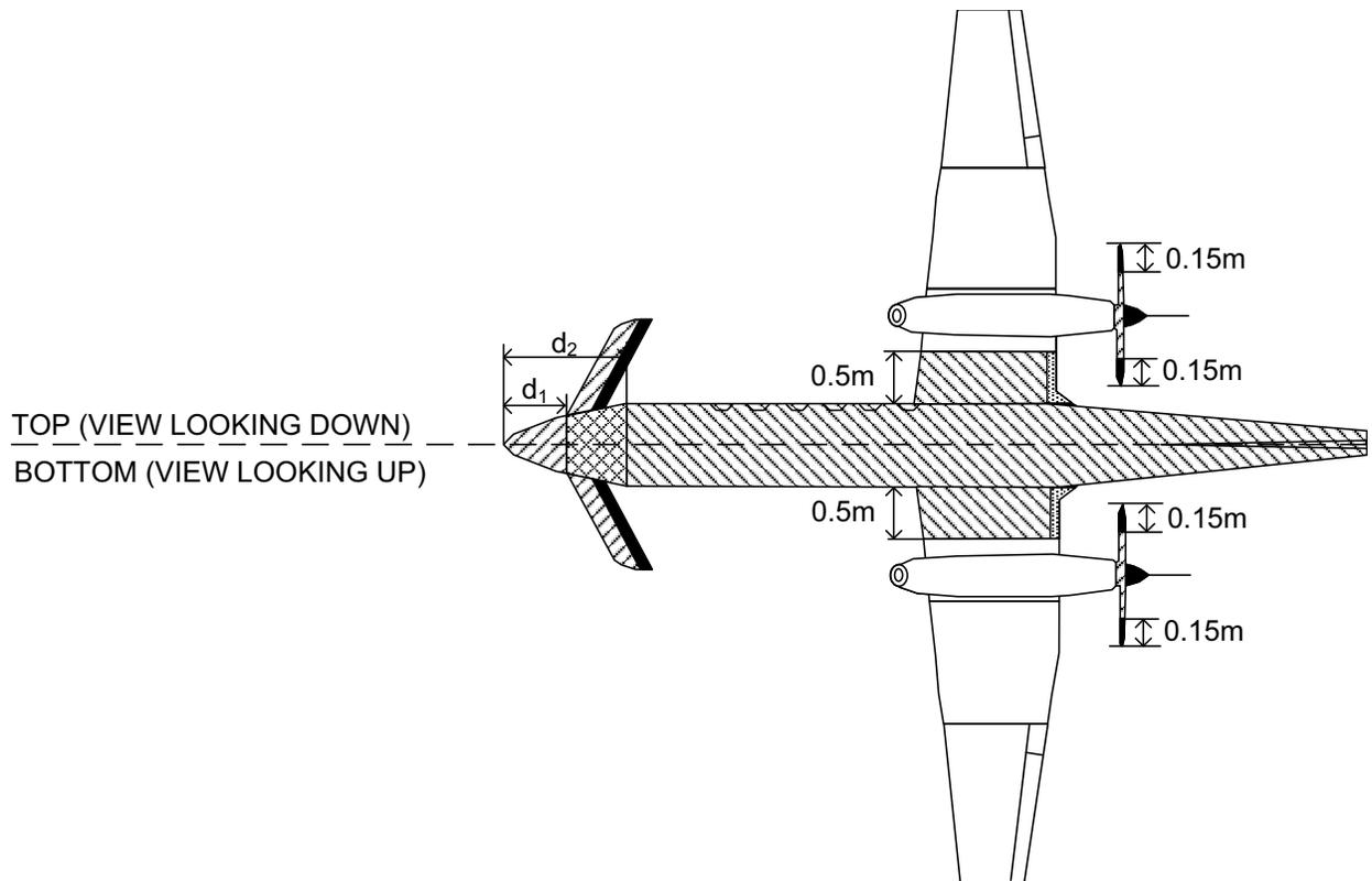
Figure F-15 Zoning for Low or High Wing Canard with Twin Rear-Facing Props
