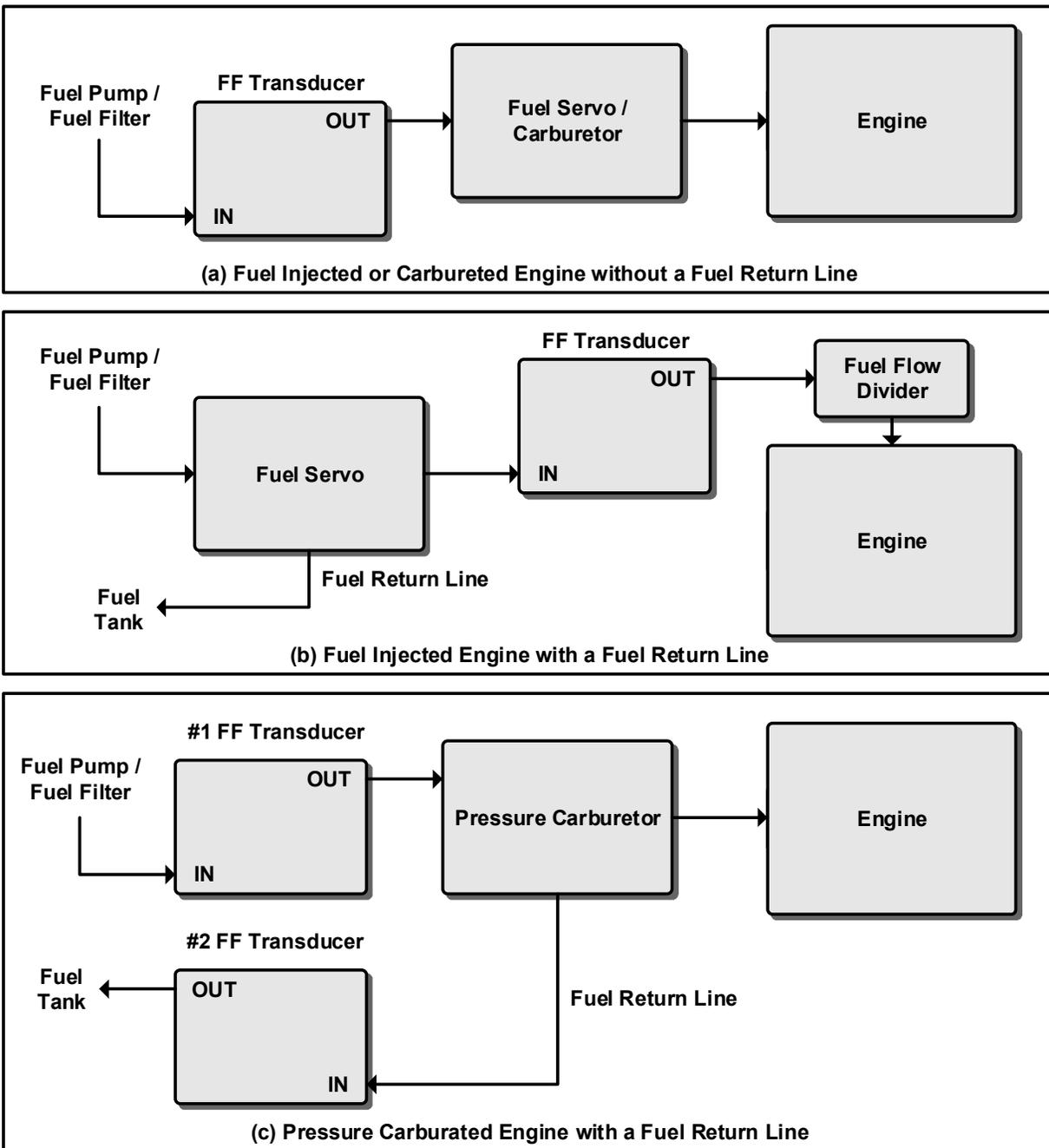
Figure 4-37 Fuel Flow Installation Configurations
