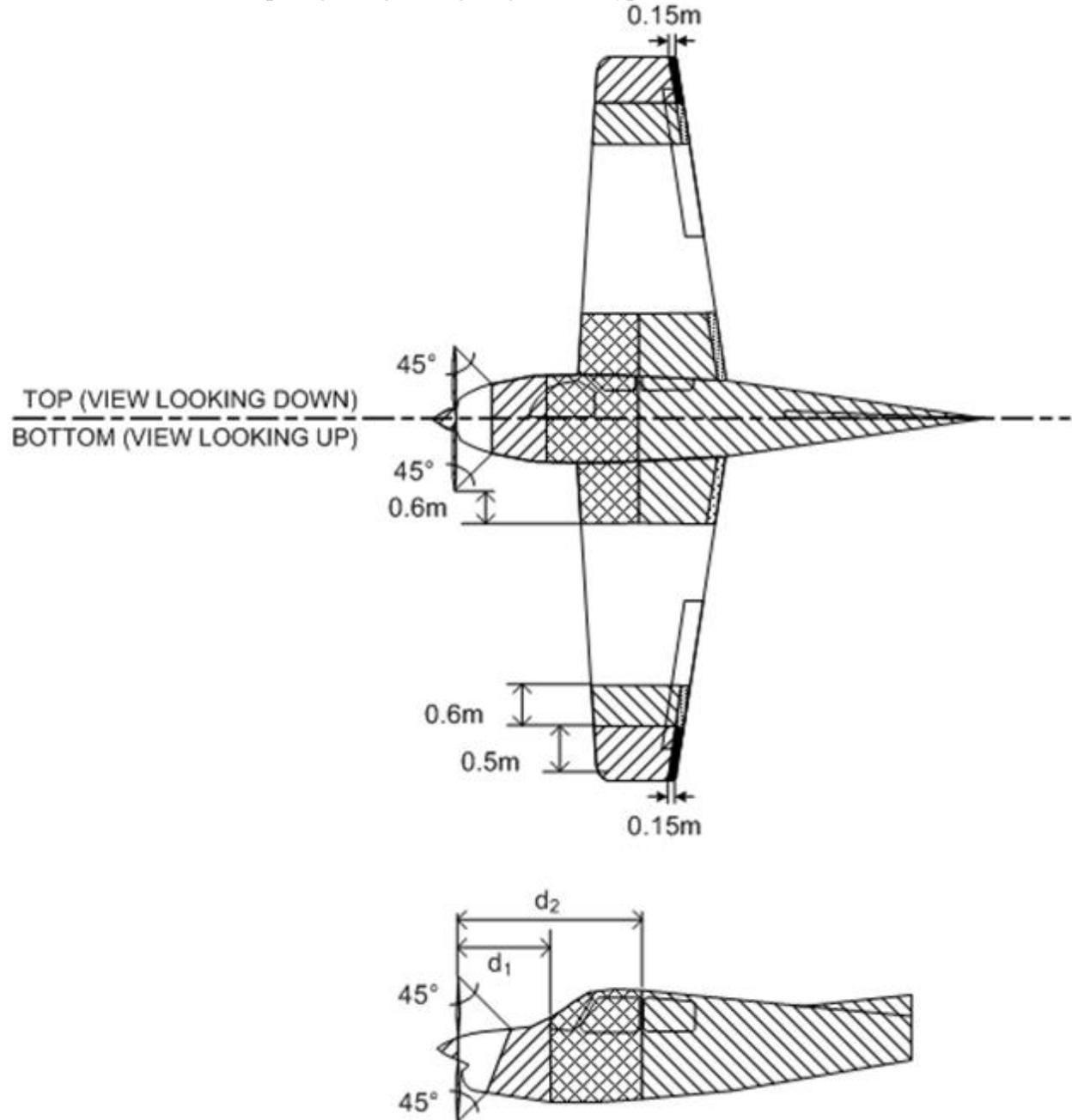
Figure F-19 Example Lightning Zoning for Single-Engine Aircraft
