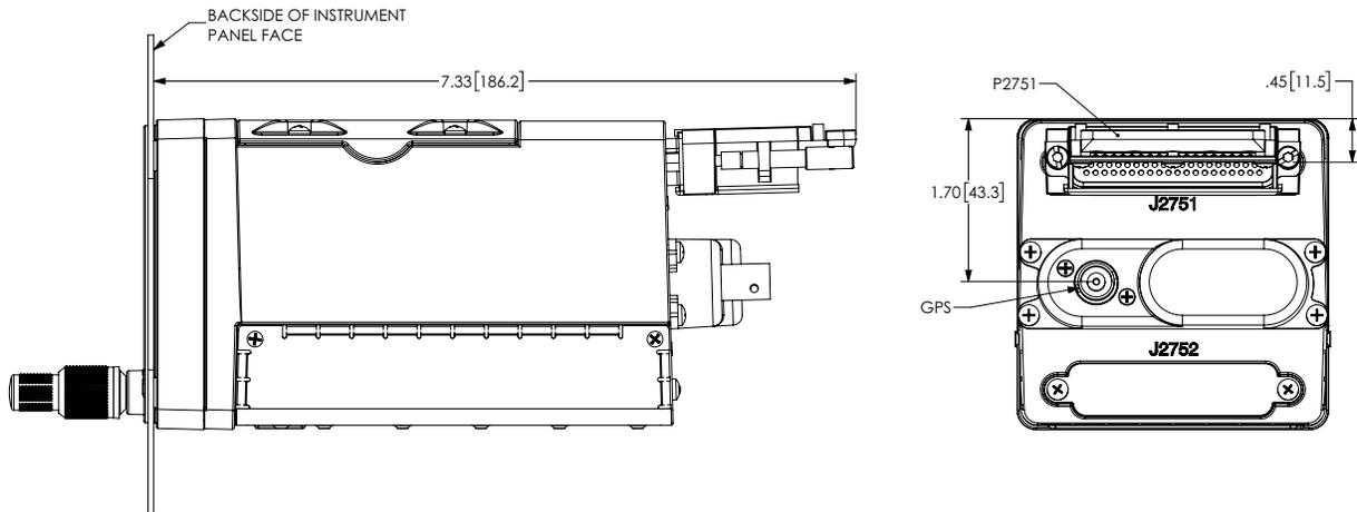
**Figure 4-6 GI 275 Multifunction Indicator Dimensions**
