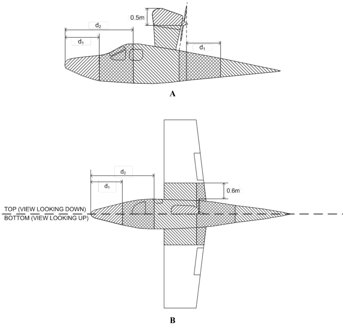
**Figure F-9 Zoning for a Single, Rear-Mounted Prop above Fuselage**
