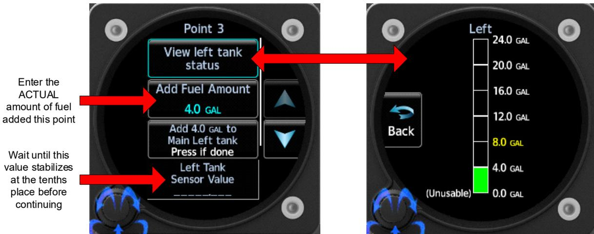
Figure 5-21 Fuel Quantity Calculation Procedure
