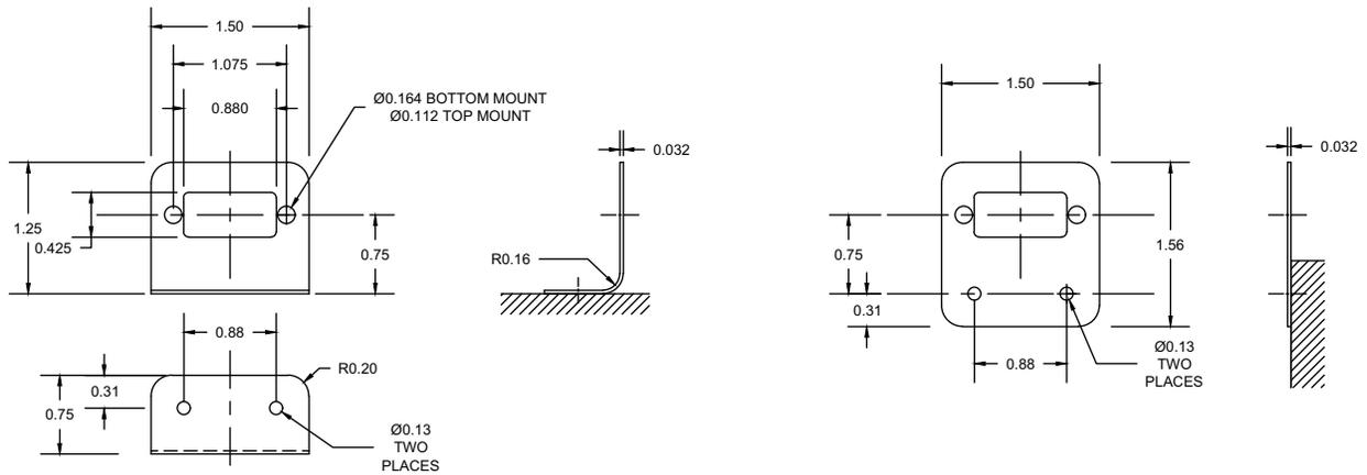
**Figure 4-43 5A Relay Bracket Examples**
