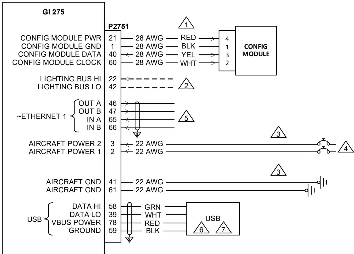
Figure B-1 GI 275 - Power, Lighting, Configuration Module, HSDB, USB Interconnect
