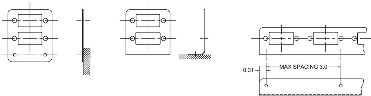
**Figure 4-44 Multiple Relay Bracket Examples**
