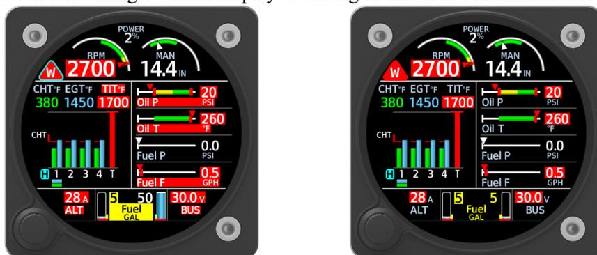
Figure E-19 Caution and Warning Alerts (Flashing and Acknowledged)
