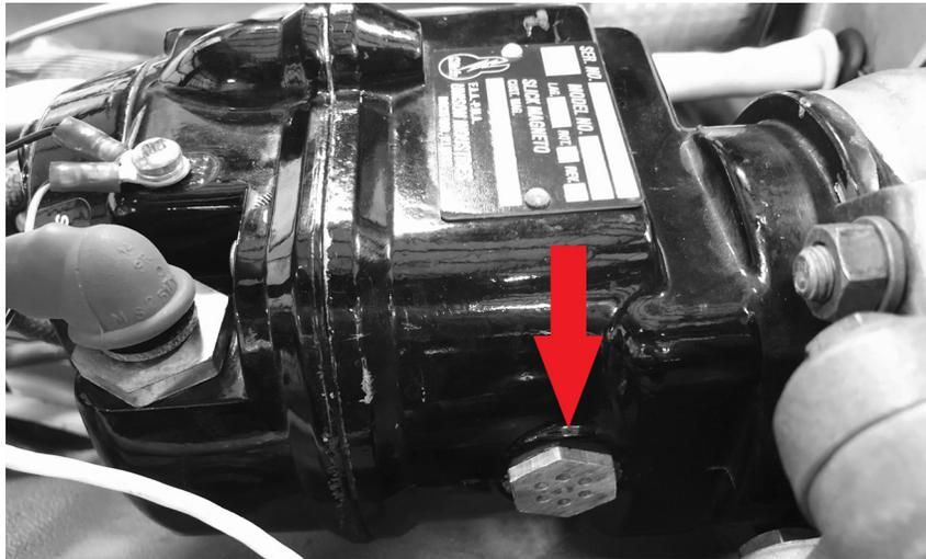
**Figure 4-41 Slick Magneto Vent Hole**
