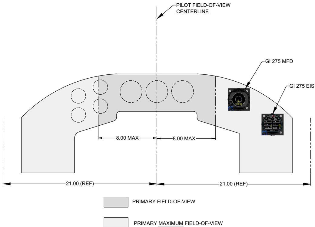
**Figure 4-5 Example of GI 275s in Non-“Six Pack” Instrument Panel (Single-Engine)**
