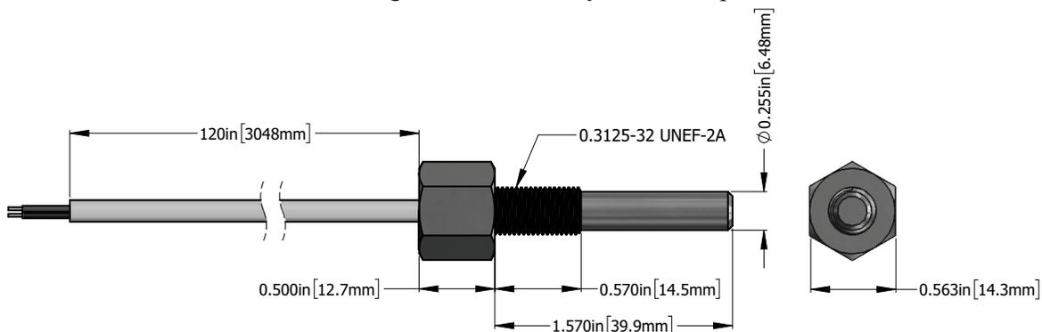
**Figure 4-25 GTP 59 OAT Probe Dimensions**
