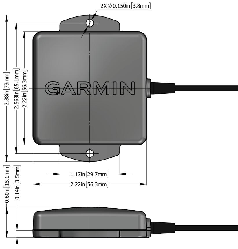
**Figure 4-22 Backup GPS Antenna Dimensions**
