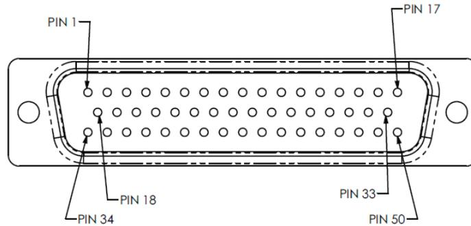
**Figure A-7 GEA 24/GEA 24B J244/P244 Connector (Looking at Unit)**
