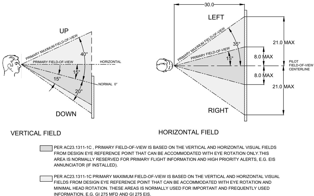
**Figure 4-2 Example of Pilot Field-of-View Installation**
