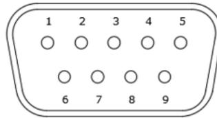
Figure A-4 GEA 24/GEA 24B J241/P241 Connector (Looking at Unit)
