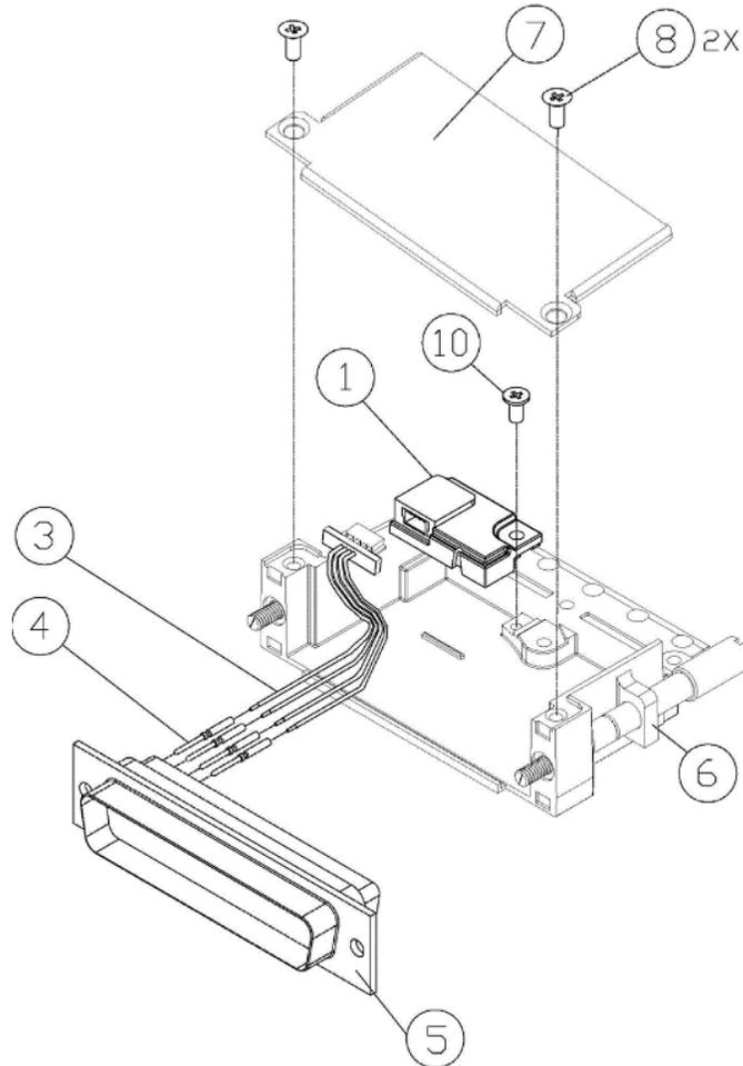
**Figure 4-21 Jackscrew Backshell Assembly
