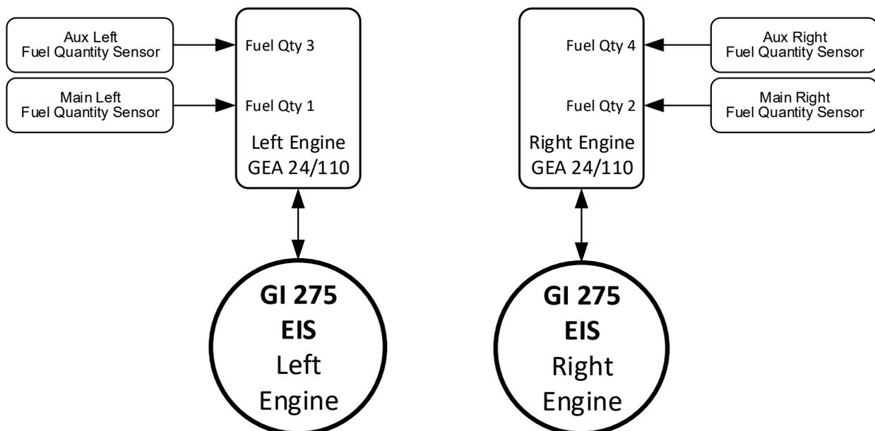
**Figure 3-4 Fuel Quantity Wiring in Twin-Engine Installations**
