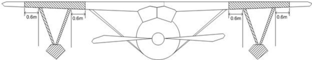
**Figure F-5 Zoning for Wings Affected by Landing Gear**
