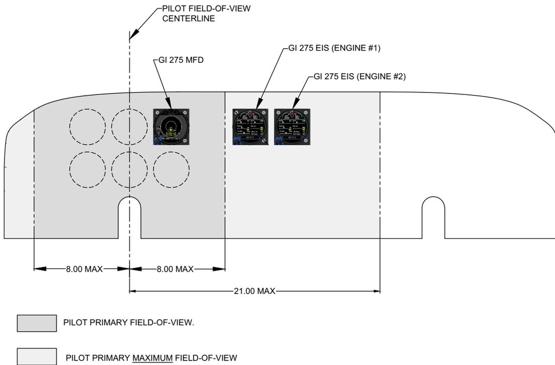
**Figure 4-4 Example of GI 275s in “Six Pack” Instrument Panel (Multi-Engine)**
