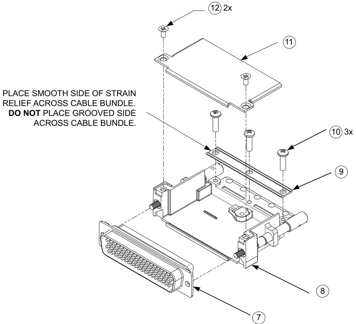
**Figure 4-19 Jackscrew Backshell and Shield Block Assembly**
