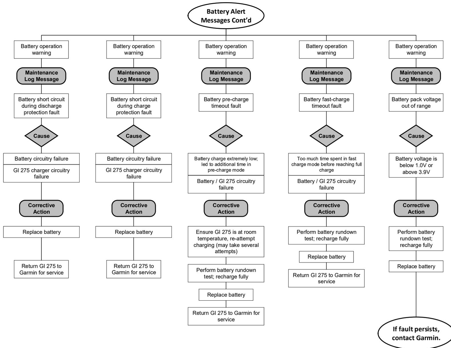
**Figure 7-2 Battery Alert Message Troubleshooting Sheet 4 of 4**
