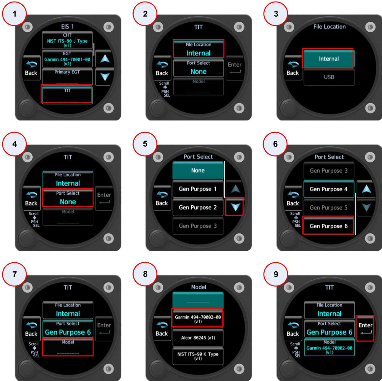
Figure 5-16 TIT Sensor Configuration Example
