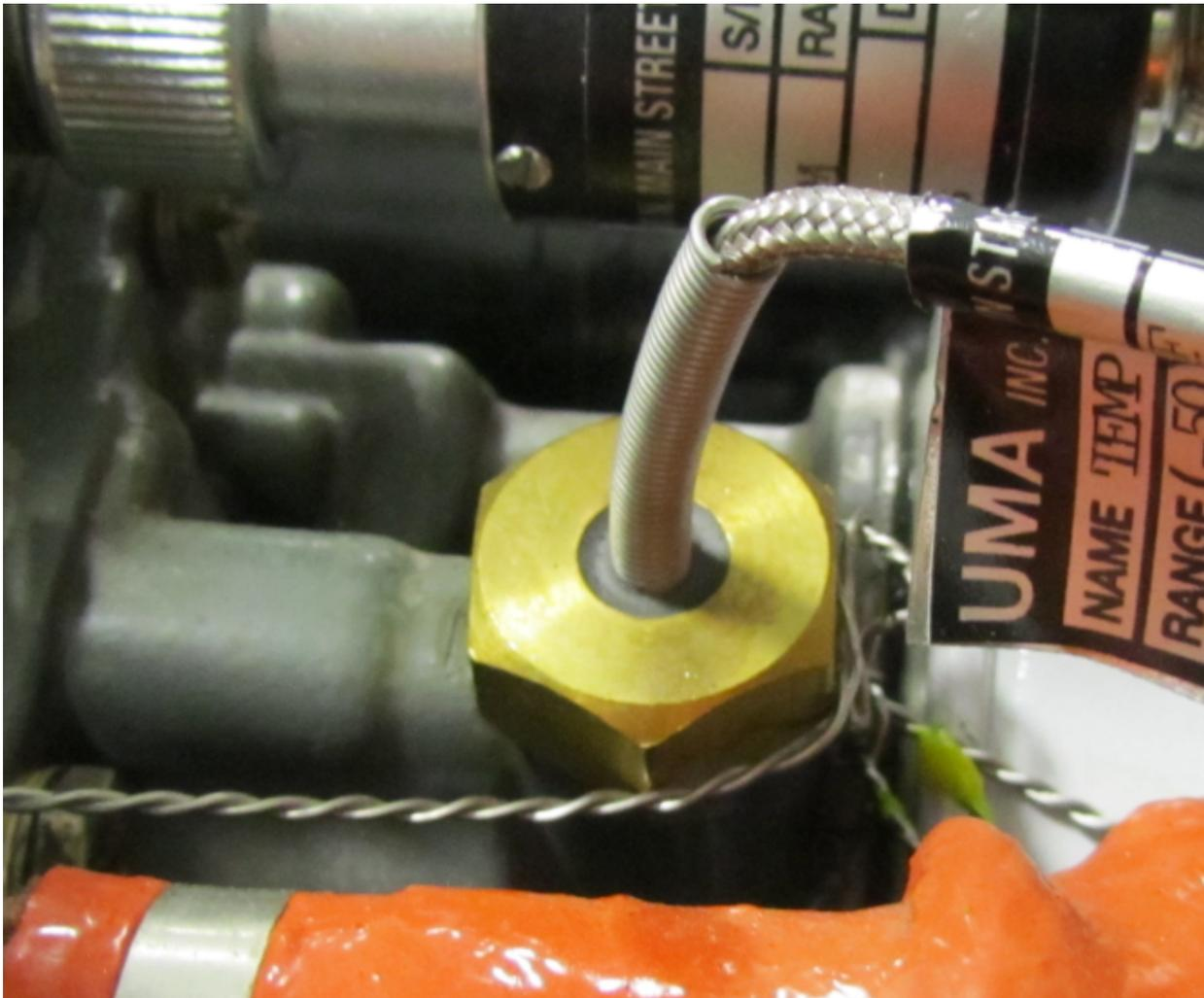
**Figure 4-33 Oil Temperature Sensor Installation Example**
