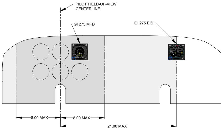
**Figure 4-3 Example of GI 275s in “Six Pack” Instrument Panel (Single-Engine)**
