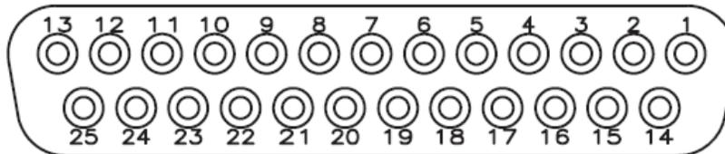
Figure A-5 GEA 24/GEA 24B J242/P242 Connector (Looking at Unit)
