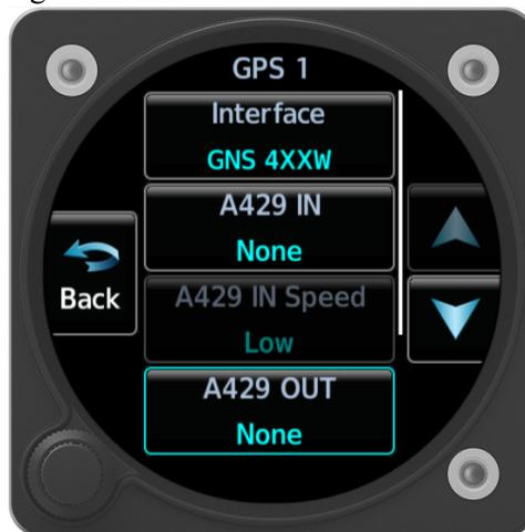
**Figure 5-4 Interface and Ports/Config Selections**
