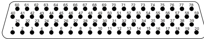
**Figure A-2 GI 275 J2751/P2751 Connector (Looking at Unit)**
