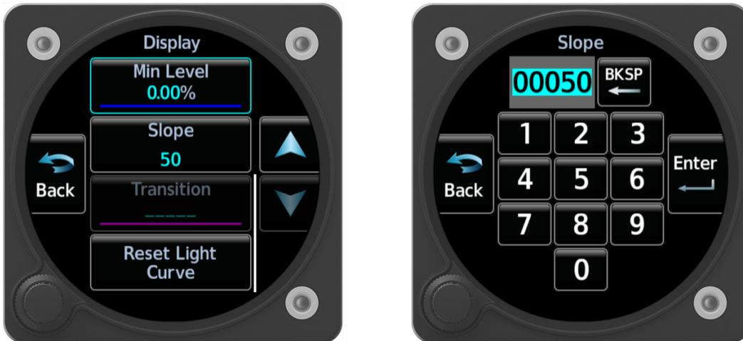
Figure 5-6 Lighting Curve Slope Configuration
