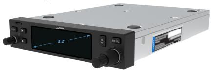
Each unit has 10 W of transmit power. Optional 16 W of transmit power is available with the purchase of a feature enablement.
