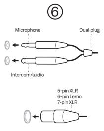
Insert the aircraft connector into the aircraft control panel.
